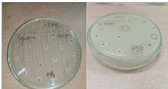
Figure-2: 'Kirby-Bauer' disc diffusion method in Mueller Hinton agar media (MHA)
